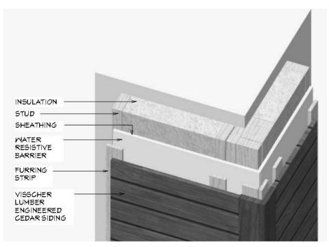
3) **Corner boards installed over siding:** Do not apply caulk or sealant at the joint between the corner boards and the siding, with this installation method.
